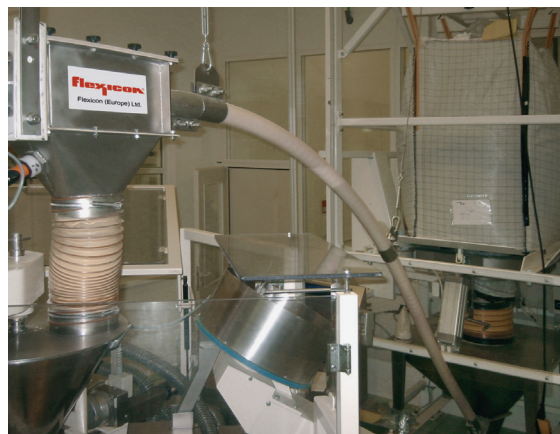
Enclosed system maintains moisture and temperature level of nutritional supplements from point of introduction to point of packaging.
