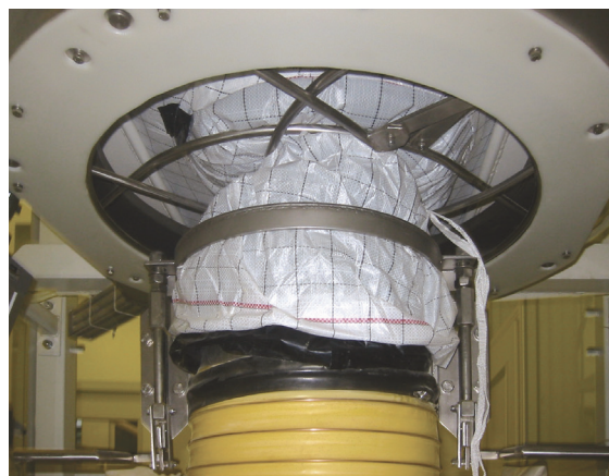
POWER-CINCHER® flow control valve (wide upper ring), SPOUT-LOCK® clamp ring (thin ring) and TELE-TUBE® telescoping tube (yellow tube) create dust-free connection between bulk bag and receiving hopper while promoting flow and permitting leak-proof retying of partially emptied bags.
