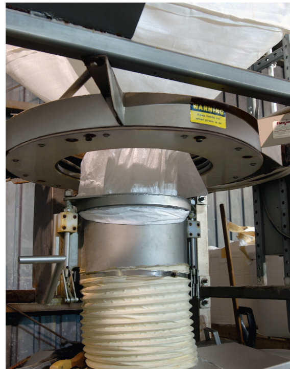
A SPOUT-LOCK® clamp ring creates a high integrity seal between the clean side of the bag and the clean side of the equipment, while a TELE-TUBE® telescoping tube maintains tension on the spout to elongate the bag as it empties and elongates, promoting complete discharge.
