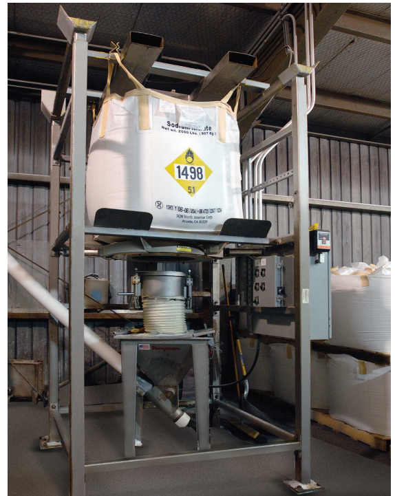
The unloader employs POP-TOP™ bag extension devices that stretch the bag into a cone shape as it empties, promoting total discharge of sodium nitrate granules.
