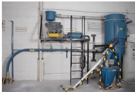
Two pneumatic lines convey PVC from the ground-floor bulk bag discharger unit to the filter-receiver on the third floor of the Oplex plant.
