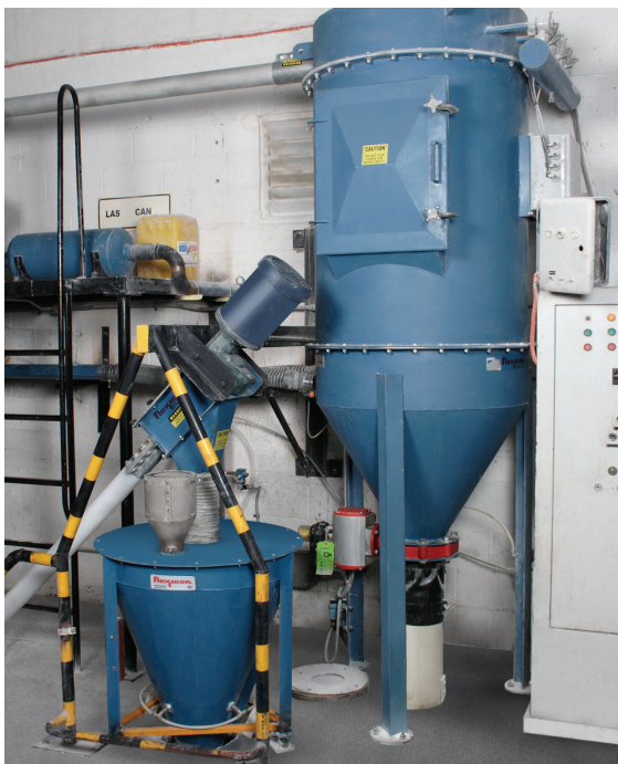
PVC from the bulk bag unloader is pneumatically transported to a 36 in. diameter (91.4 cm) filter-receiver and hopper on the third floor of the Oplex plant. The flexible-screw conveyor empties calcium carbonate into the smaller weigh hopper. Both ingredients are then gravity fed to the mixer on the floor below.
