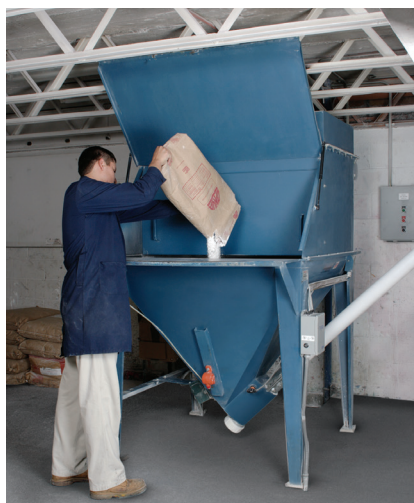
Worker loads calcium carbonate additive into bag-dump station on the second floor of the Oplex plant. The flexible screw conveyor, located on the right, transports the additive 30 ft (9 m) to a weigh hopper on the third floor.
