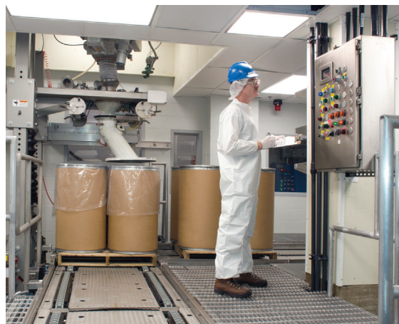
PLC communicates with weigh-filler scale to regulate product flow into each drum and shut down on reaching a pre-set weight. Four drums await filling as four are about to exit the room. System improves product output, worker safety, and quality control.
