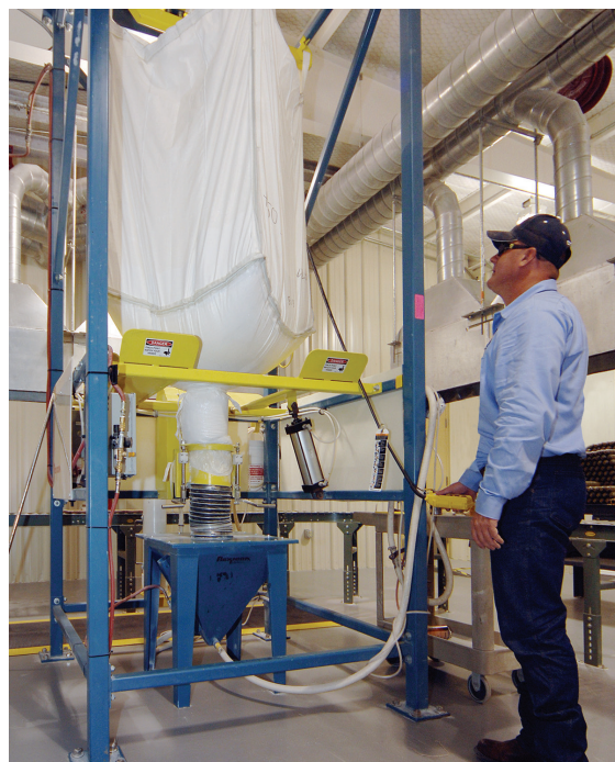
Sodium-bicarbonate powder is transferred from a Flexicon bulk bag unloader, into a hopper and through a hose to refill canisters on conveyor line. TELE-TUBE® telescoping tube, between bag outlet and hopper, elongates the partially empty bag to prevent dead spots and flow restrictions. FLOW-FLEXER® bag activators (yellow plates) raise and lower bottom edges of the bag to promote total evacuation.
