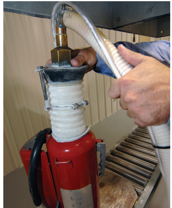
Canister, ready for refill, is fitted with two hoses: one for carbon dioxide or nitrogen, and one for sodium bicarbonate powder.
