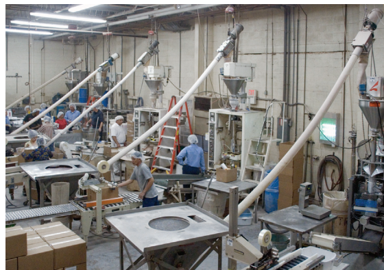
Eight flexible screw conveyors feed spice blends to packaging machines. Three conveyors (not shown) are dedicated to dry cappuccino mix.
