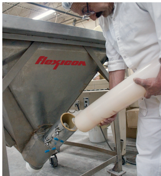
Operator quick-disconnects conveyor tube before moving it to the cleaning area.
