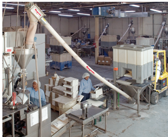
Forklift operator sets tote atop 8 cu ft (2.4 sq m) hopper from which a 15 ft long (4.6) flexible screw conveyor transports blends to packaging machine.
