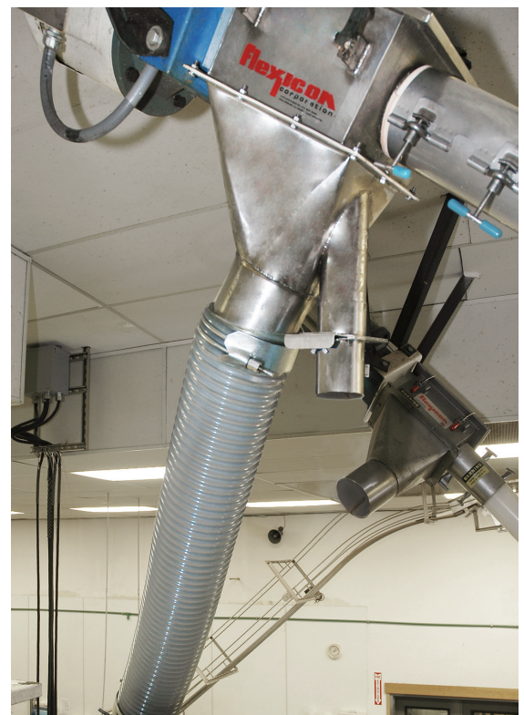
Operator dumps cashews into hopper as flexible screw conveyor transports them to the grinding process.
