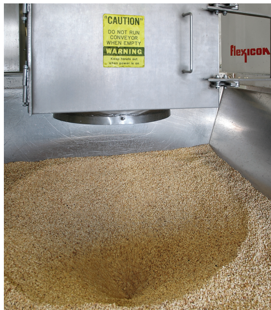
In the roasting room, bulk bag discharger empties almonds into hopper as a flexible screw conveyor transports them to the roaster. A POWER-CINCHER® flow control valve cinches the bag spout concentrically, allowing leakproof retying of partially empty bags.
