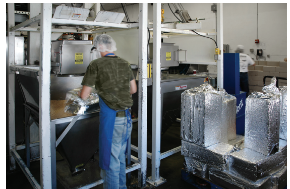
Operator dumps cashews into hopper as flexible screw conveyor transports them to the grinding process.
