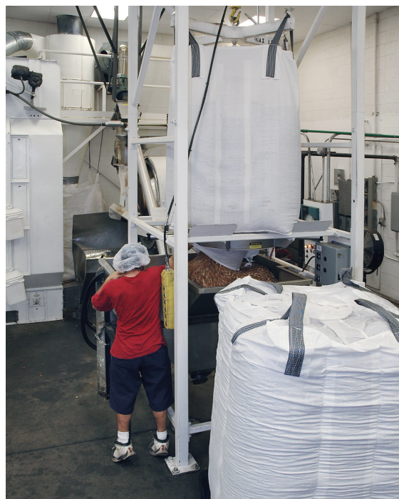
In the roasting room, bulk bag discharger empties almonds into hopper as a flexible screw conveyor transports them to the roaster. A POWER-CINCHER® flow control valve cinches the bag spout concentrically, allowing leakproof retying of partially empty bags.
