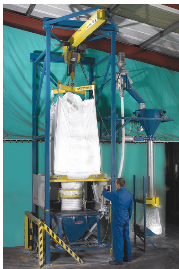
A bulk bag is mounted in the frame, ready to discharge clay into the receiving hopper via the TELE-TUBE® assembly.
