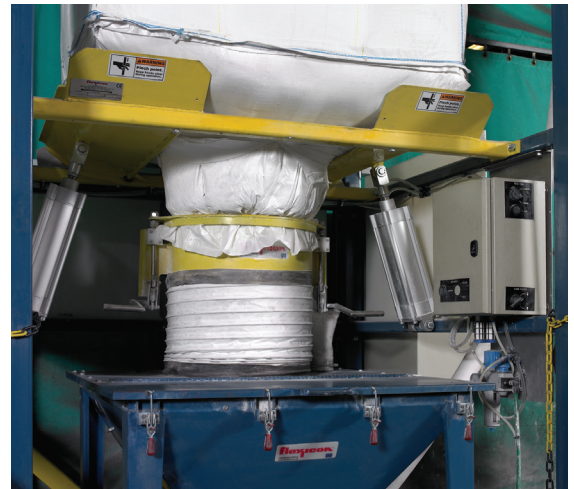
The SPOUT-LOCK® clamp ring and TELE-TUBE® telescoping tube allow a quick, dust-tight connection between the bag spout and the hopper and elongate the bag as it empties, thereby promoting flow.
