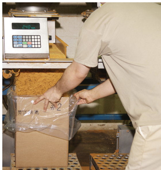
On the packaging line, product destined for restaurants is loaded into a box by a vibratory feeder trough. An operator removes the box from the scale when it reaches the preset weight.
