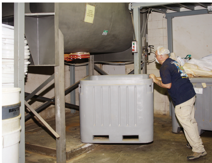
A batch of product is unloaded from a paddle mixer into a 1,500 lb bulk bag that is draped inside a tote bin.
