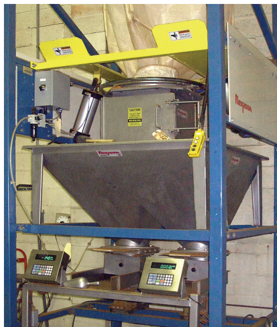
The bulk bag discharger empties a 1,500 lb bag of product into a hopper that feeds two packaging lines.
