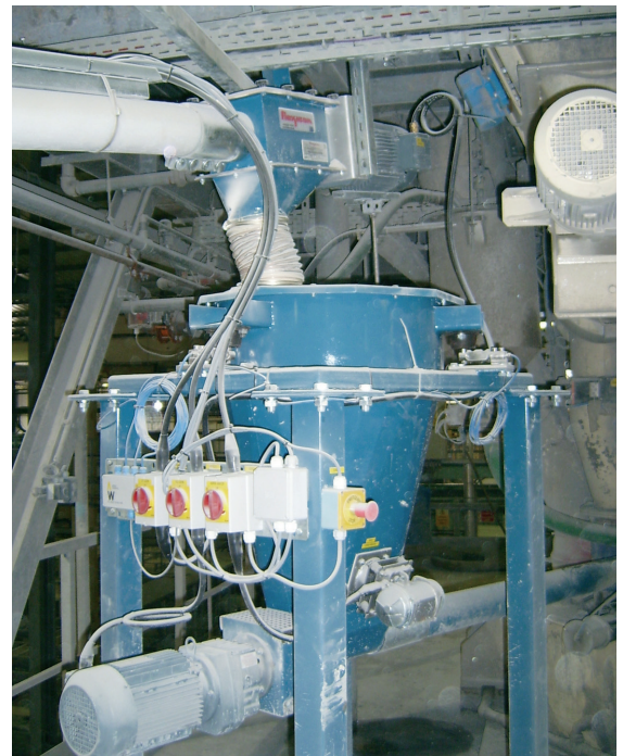
The upper flexible screw conveyor transfers aluminum powder from the bag dump station to the top of a weigh hopper, while the conveyor below feeds weighed batches to the blender.
