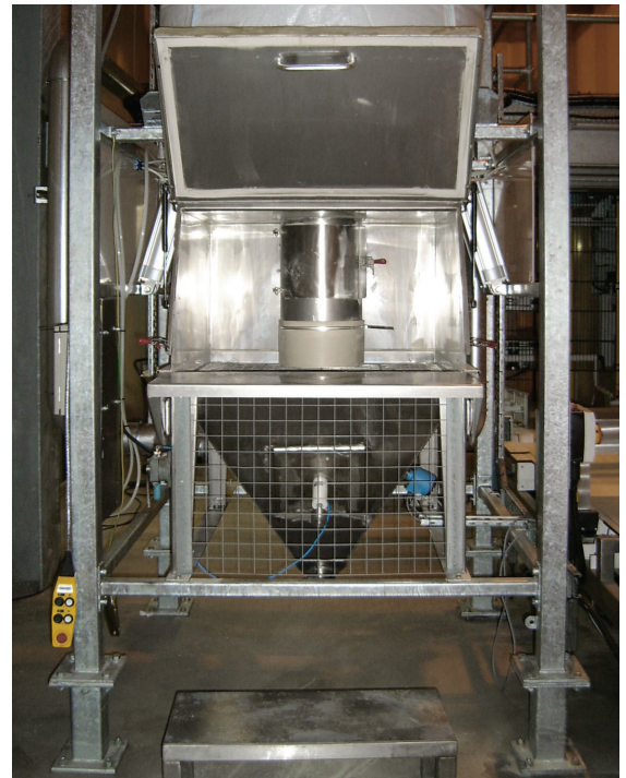
Opening a door on the hopper intake chute of the bulk bag discharger frame exposes the bag spout.
