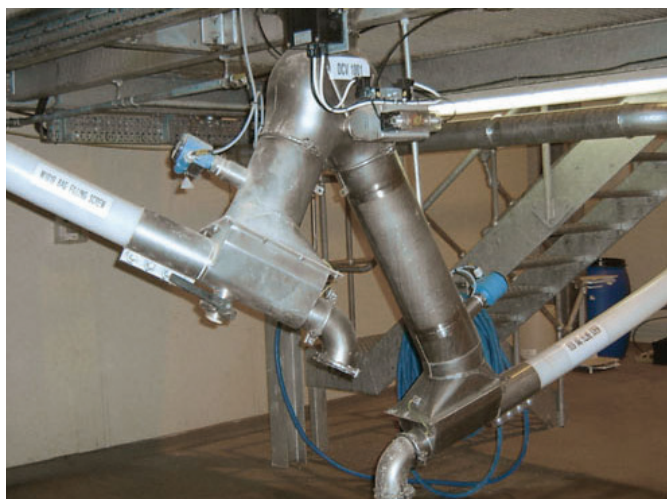
Two flexible screw conveyors transport powdered malt from the cone mill to the bagging line or, in the event of a bagging line shutdown, to a bulk bag filler.
