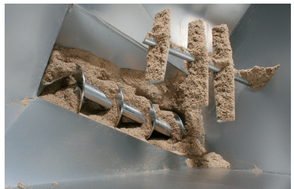
A rotating agitation device protruding from the hopper wall promotes uninterrupted flow of material into the intake adapter of the flexible screw conveyor.
