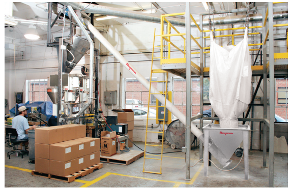
General views of the RitePak operation. Above shows a bulk bag being loaded into the floor hopper, from which the product is moved by the flexible screw conveyor to the blender at the upper left.
