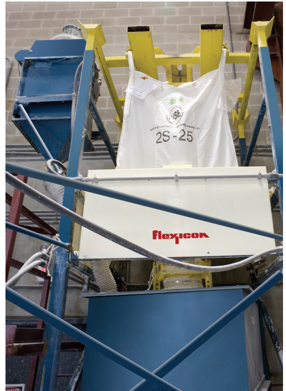
A BAG-VAC® dust collector, mounted on the bulk bag unloader frame, vacuums displaced air and dust, and collapses empty bags dust-free prior to tie-off and removal. The bulk bag is supported in a lifting frame.
