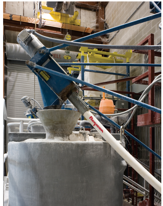
At the flexible screw conveyor's discharge end, DE flows through a transition adapter into the 300 gal (1136 l) tank where the DE is put in suspension with water.
