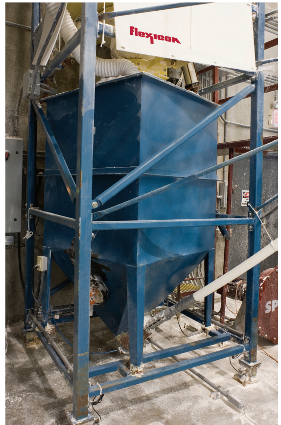
A BAG-VAC® dust collector, mounted on the bulk bag unloader frame, vacuums displaced air and dust, and collapses empty bags dust-free prior to tie-off and removal. The bulk bag is supported in a lifting frame.
