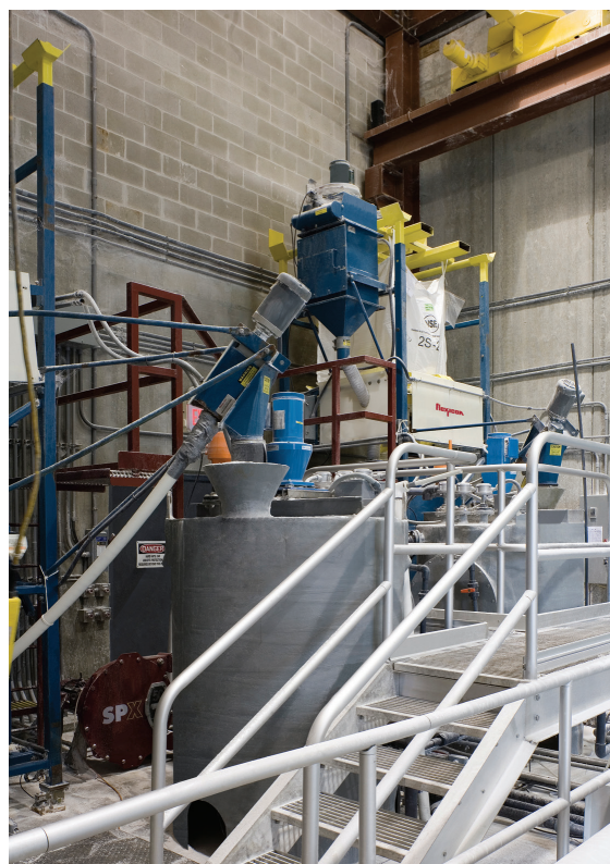
Two bulk bag unloaders unload and transfer 4000-6000 lb (1814-2722 kg) per day of diatomaceous earth (DE) for Tampa Bay desalination plant's DE filtration system. The crane deposits a lifting frame holding the bulk bag onto the unloader frame.
