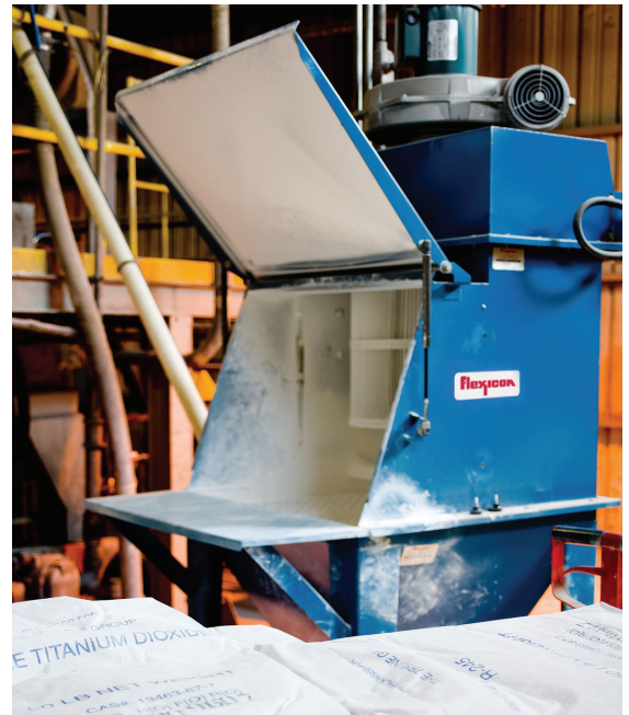
25 lb (11 kg) bags of titanium dioxide, a dusty powder, are manually emptied into the bag dump station, which includes dust collection, and a support tray for opening bags.
