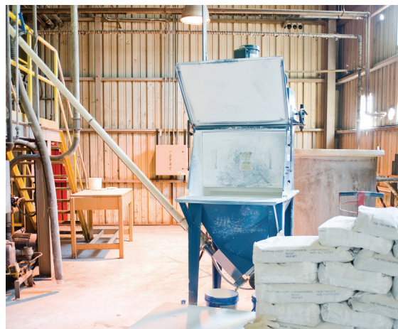
A 25 ft (7.6 m) long flexible screw conveyor transports titanium dioxide to the mixer on the mezzanine. The conveyor employs a flexible screw with specialized geometry for moving the non-free-flowing material.
