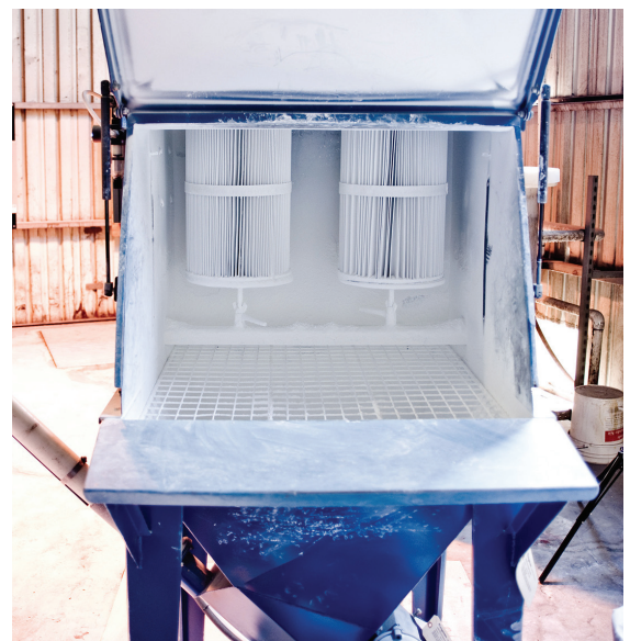
The bag dump station's support tray provides a work surface to open bags prior to dumping. A vacuum fan pulls dust onto the filter cartridges, while a pneumatic vibrator and an agitator promote flow of the difficult-to-move powder toward the flexible screw conveyor's inlet at bottom.
