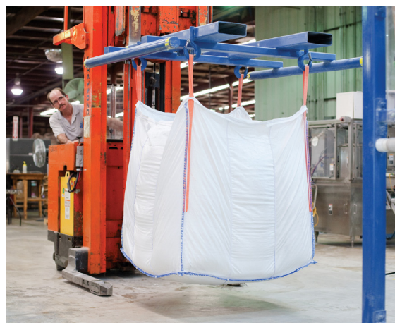
Operator attaches bulk bag to lifting frame and forklift-loads the frame and bag onto the bulk bag discharger.
