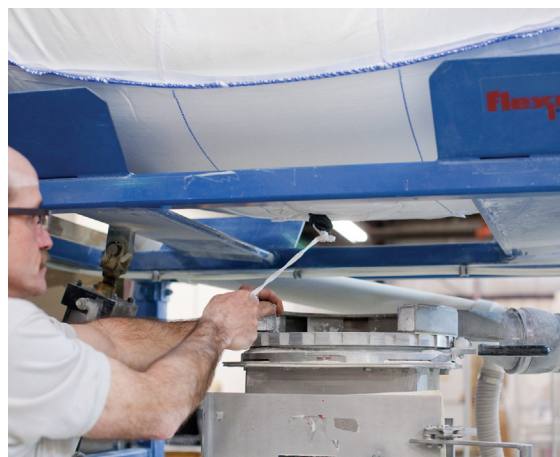
Once the bag spout is pulled through the iris flow control valve, the operator closes the valve, unties the spout drawstring, and slowly opens the valve
