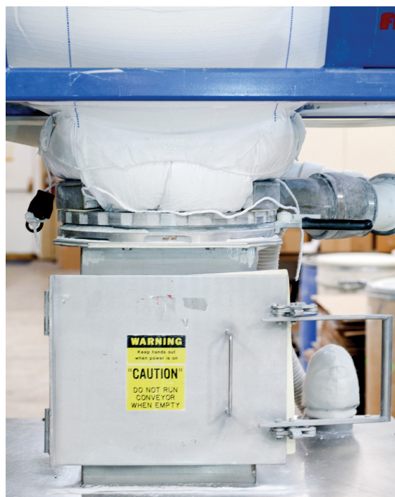
Operator attaches bulk bag to lifting frame and forklift-loads the frame and bag onto the bulk bag discharger.
