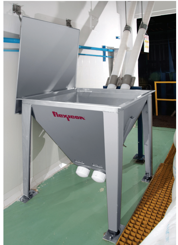
Footprint of the system is reduced by the curvature of the flexible conveyors, which are charged by a dual intake adapter at base of the hopper.
