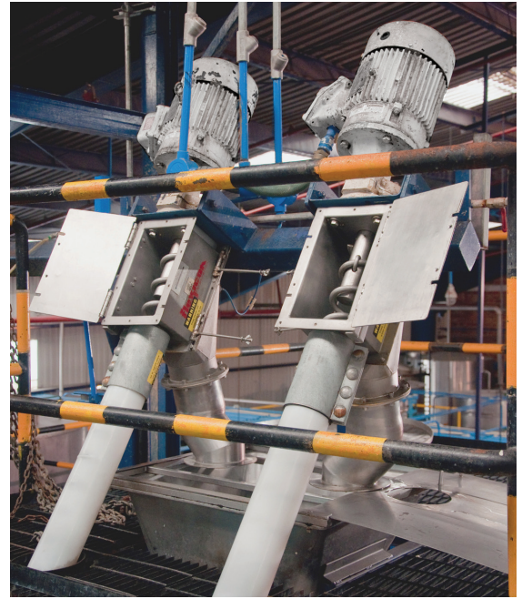
Open cleanout doors reveal the flexible screws, which are driven by electric motors at the discharge end.
