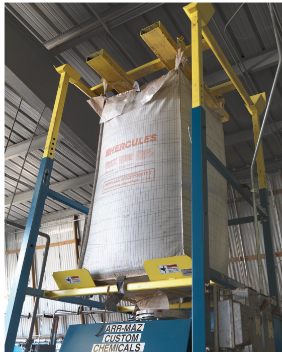
At top of the unloading frame, POP-TOP® bag extension devices raise and elongate the bulk bag, promoting flow through the bag spout. At bottom, pneumatically actuated FLOW-FLEXER® plates raise and lower opposite bottom sides of the bag, loosening material and directing it through the bag spout.
