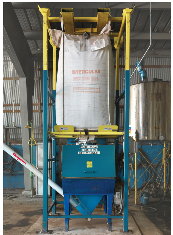
Cradle at top of the bulk bag unloader supports the removable bulk bag lifting frame. An iris valve between the bag spout and manual dumping hood controls the rate at which the bulk resin enters the hopper.
