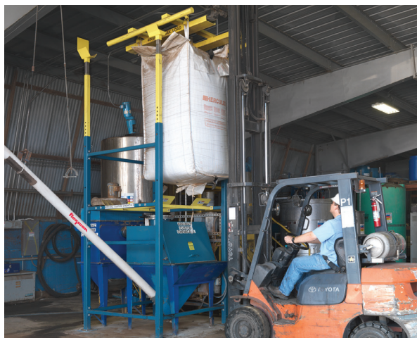
Forklift operator positions bag lifting frame on top of the bulk bag unloader. The 22 ft (6.7 m) long flexible screw conveyor transports resin from the bag dump hopper into a 6000 gal (22,713 l) tank.
