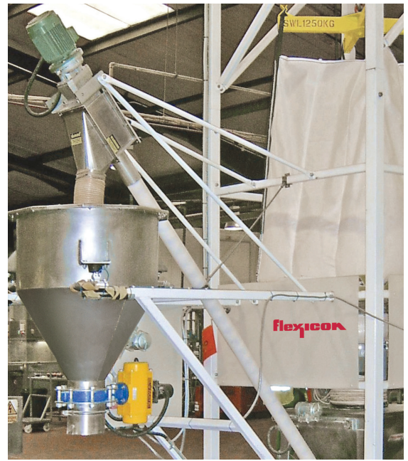
Bulk bag weigh batching system conveys dry ingredients from bulk bag to a gain-in-weight hopper that discharges into mobile wet mixing vessels.
