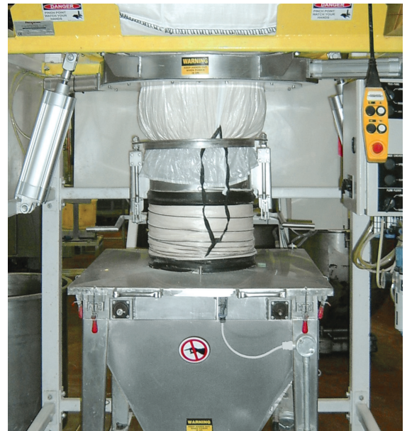
The SPOUT-LOCK® clamp ring and TELE-TUBE® telescoping tube create a fast, dust-tight connection between the bag spout and receiving hopper.
