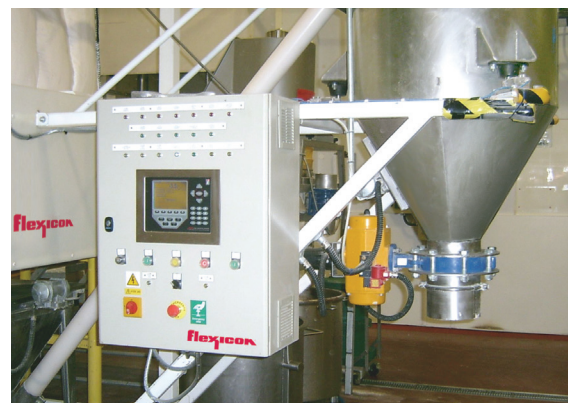
Control system with full function weighing indicator starts and stops conveyor, and actuates a slide gate.
