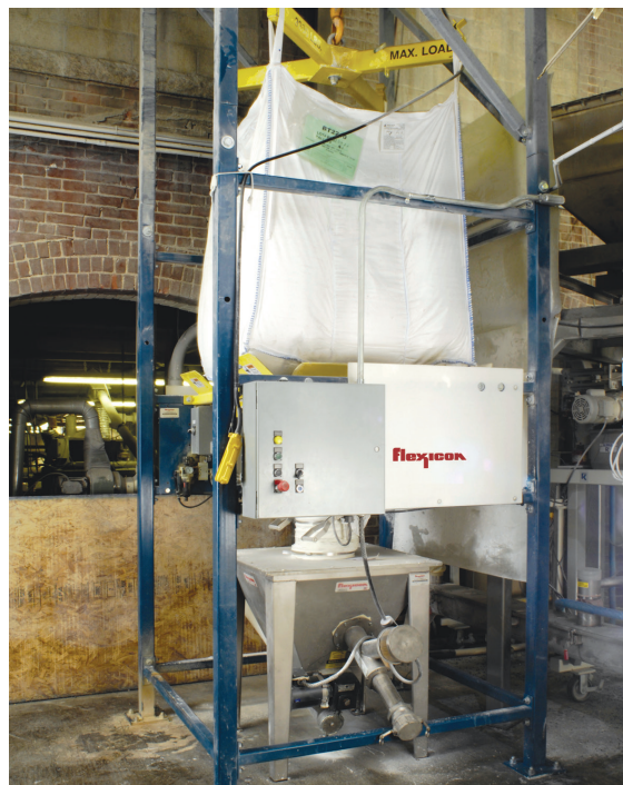
Flexibility of conveyor line routing allowed The Plastics Group to position two Flexicon bulk bag dischargers in restricted spaces, eliminating the need for a costly network of pneumatic lines.
