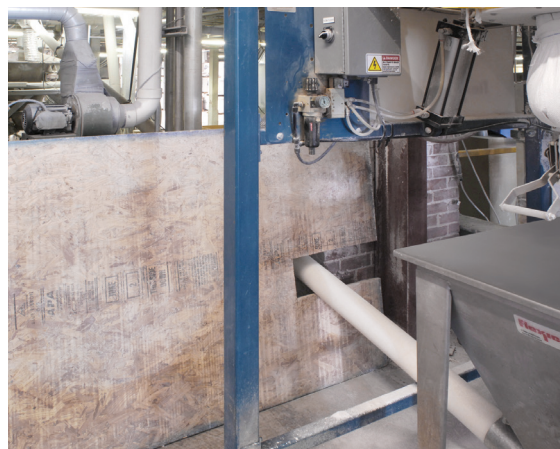
The 4.5 in (115 mm) diameter flexible screw conveyor from the second bulk bag discharger passes through a wall to reach the additive hopper on the extruder, overcoming space limitations.
