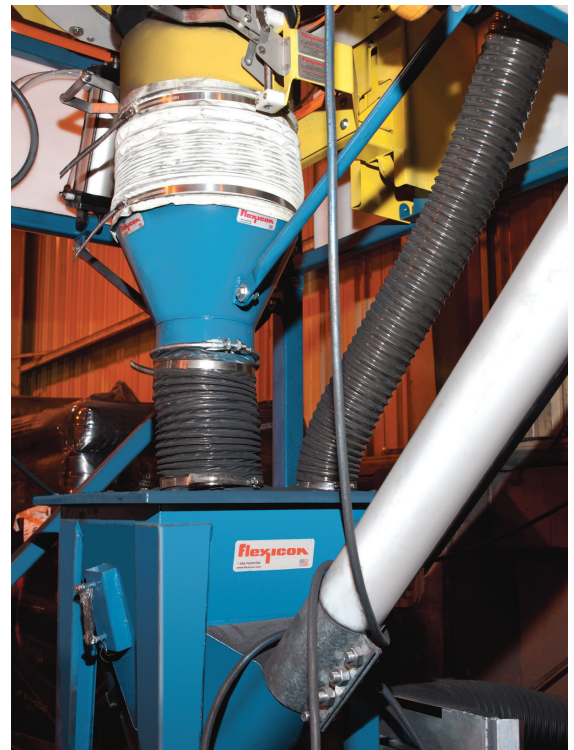
The bulk bag discharger, hopper and flexible screw conveyor from Flexicon fully contain carbon black pellets, preventing dust from entering the plant environment. A SPOUT-LOCK® clamp ring forms a sealed connection between the bag spout and the TELE-TUBE® telescoping tube, which keeps the bag taut as it empties/elongates, promoting discharge. The sealed system is vented through the black hose to a BAG-VAC® dust collector that contains displaced dust and collapses empty bags, eliminating dust caused when bags are flattened manually.
