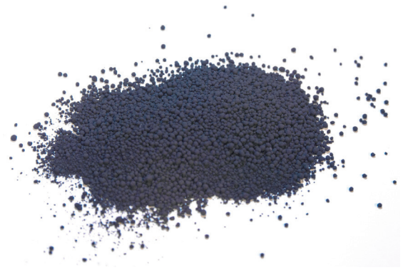
Dust is created as 1-3 mm diameter carbon black pellets rub together.
