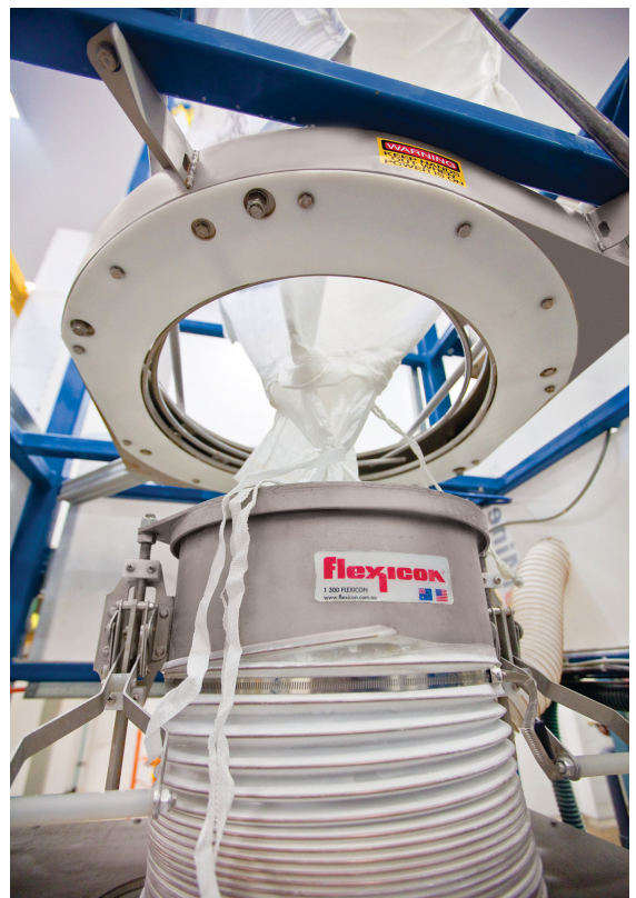
Double wall TELE-TUBE® telescoping tube provides extra protection against dust leakage during transfer from the bag. Tube is secured to the bag spout by a SPOUT-LOCK® clamp ring that creates a dust-tight seal.
