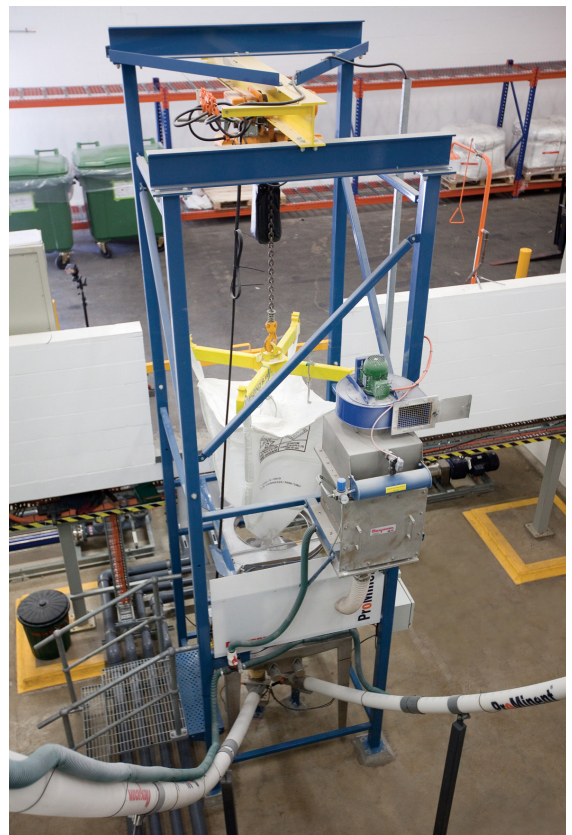
Powder remains enclosed from the time it is received until it enters the mixing tanks. The BAG-VAC dust collector, on the right of discharger frame, prevents any dusting during bag loading and removal and collapsing of empty bags.
