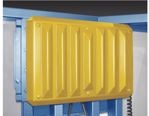
Hydraulic conditioning plates on opposing sides of the bag loosen the material.
