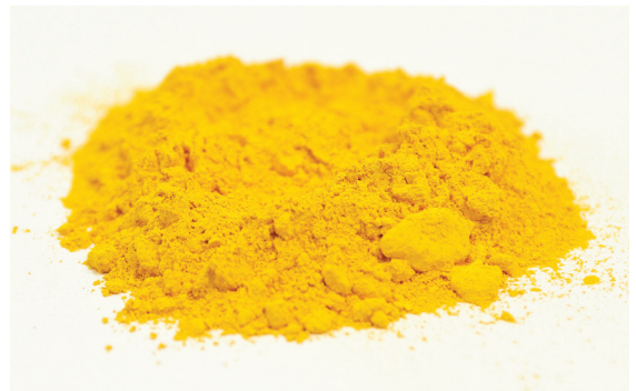
Offset inks begin as CMYK (cyan, magenta, yellow, key [black]) pigments. Each powder is transferred by its corresponding-colored bulk bag discharger system.
