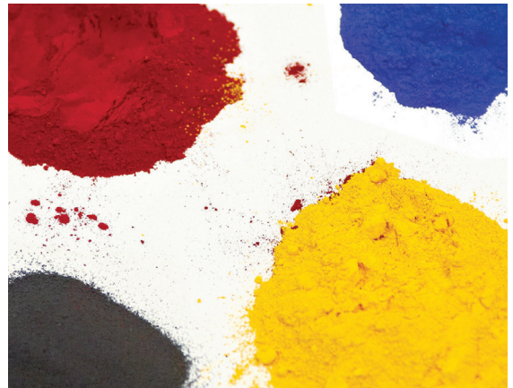
Offset inks begin as CMYK (cyan, magenta, yellow, key [black]) pigments. Each powder is transferred by its corresponding-colored bulk bag discharger system.
