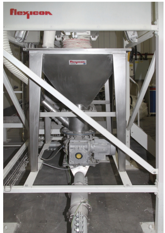
Raw material is gravity fed from the hopper through a rotary airlock with a pick-up adapter for discharge into a pneumatic line leading to a tanker truck loading bay.
