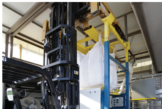
Forklift positions the bulk bag lifting frame onto the cradle atop the discharger frame.
