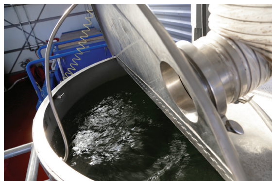
Diatomaceous earth (D.E.) aids in filtration to remove solids from crushed and fermented grapes in 300 gal (1136 l) steel tanks before aging of the wine.
