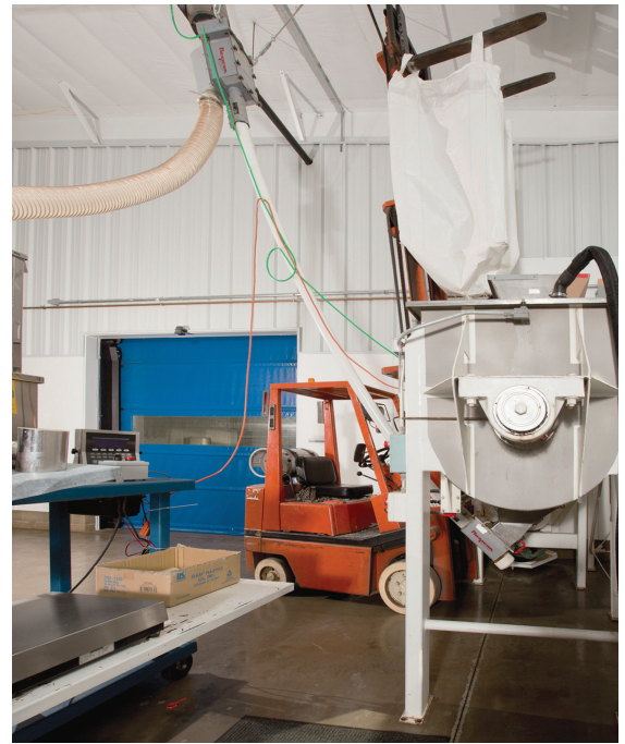
A bulk bag containing whey powder is discharged into a ribbon blender, where it is mixed with smaller amounts of colostrum, vitamins and minerals. The flexible screw conveyor, fully enclosed, moves the mixture to the packaging machine.
