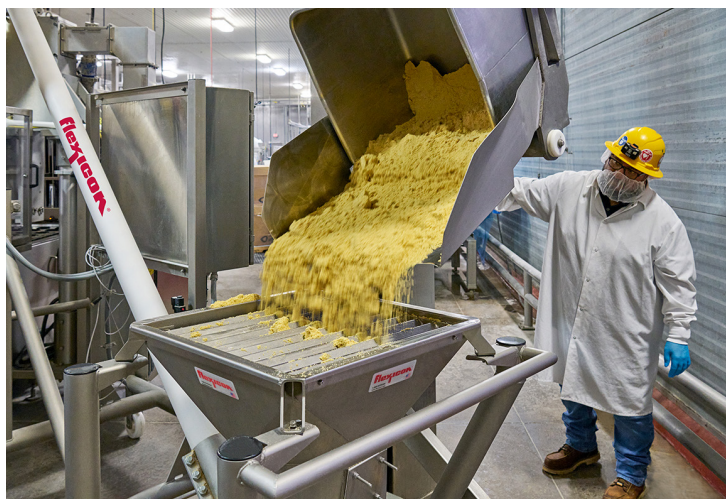
Operators wheel the filled tote over to a mechanical tipper, which unloads the contents into the conveyor's hopper.
