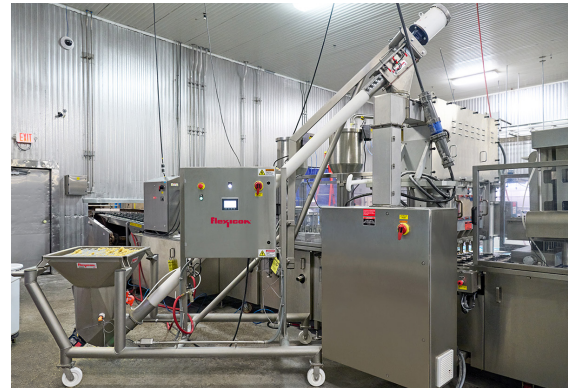
Designed for mobility within the plant, the castor-mounted Flexicon system includes a steep-walled hopper, level sensor, and vibratory sidewall activation device to promote the flow of sticky materials.
