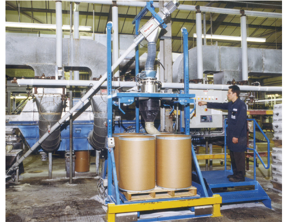
Polymer resins are safely conveyed and accurately dispensed into kegs, boxes or bulk bags using this self-contained Flexicon Automated Filling Station
