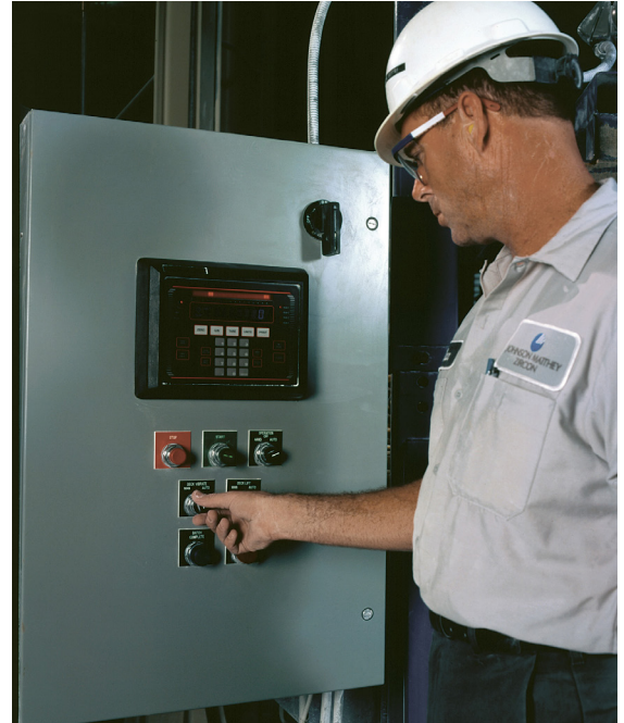
Operator inputs settings on frame-mounted control panel. Load cells transmit gain-in-weight information to controller which actuates a rotary valve, filling bags to +/-1% accuracy.
