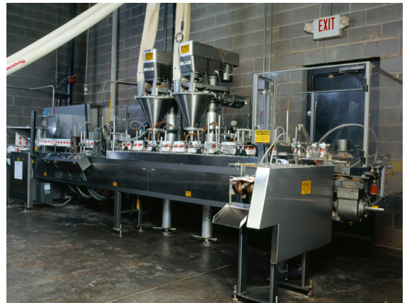
Recently installed twin horizontal form/fill/seal machines for institutional pouches accept product from the conveying tubes of flexible screw conveyors.
