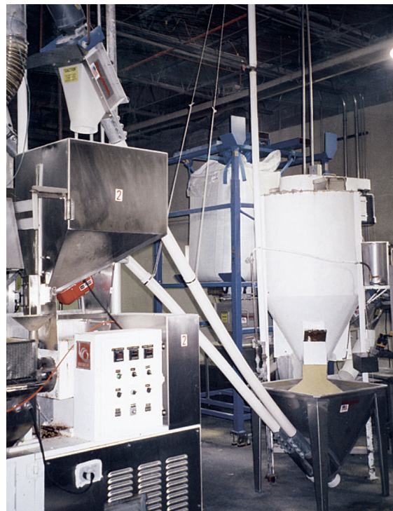
Bulk bag discharger with flexible screw conveyor is mounted on load cells that transmit loss-of-weight information to a controller which stops the conveyor once the target batch weight is discharged.
