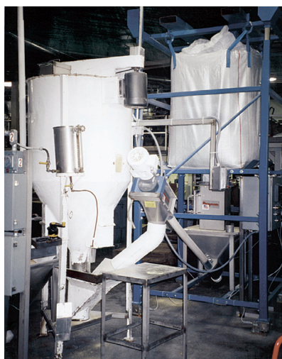
Bulk bag unloader with 2000 lb bag of cornmeal discharges into hopper equipped with flexible screw conveyor which transports the material to a vertical blender where it is moisturized.
