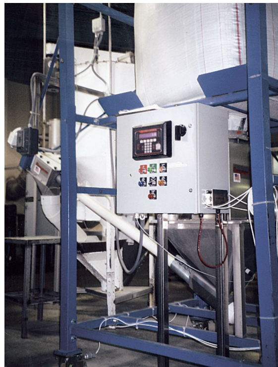
Moistened cornmeal discharged from vertical blender into floor hopper is transported by the Flexicon flexible screw conveyors that feed two extruder surge hoppers.
