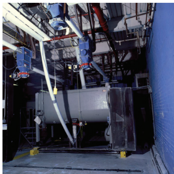
Ingredients are fed into a ribbon blender by a flexible screw conveyor through a discharge transition adapter.
