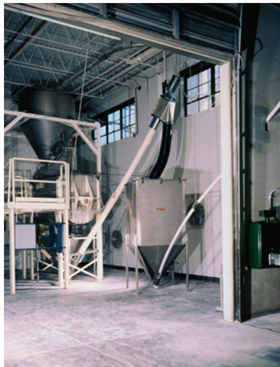
The larger flexible screw conveyor loads product into a 100-cubic foot surge hopper, freeing the blender's discharge hopper to receive additional product.
