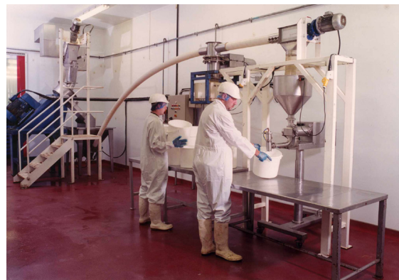
From pulverizer (left), puree is transferred through a second flexible screw conveyor to two gate valves from which line-end operators fill buckets.
