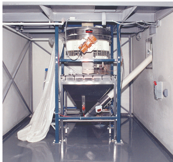
Powdered milk emptied from bags into bag dump station flows through 48 in diameter circular vibratory screener into Flexicon floor hopper, from which flexible screw conveyor, at a 45-degree incline, transports the powder to form-fill-seal machine in adjacent room.
