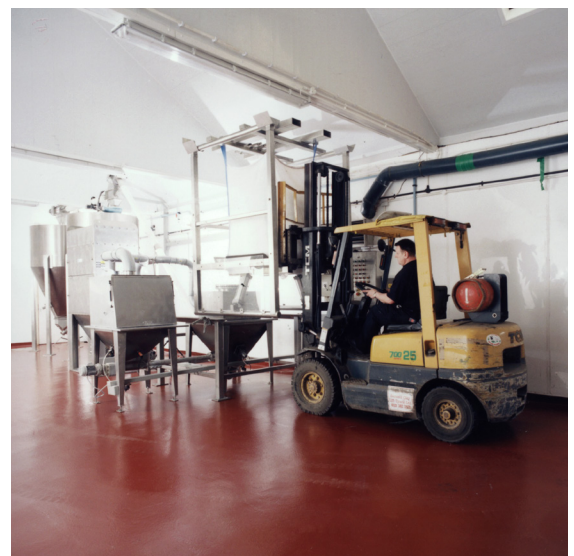
Fork lift truck negotiates intermediate frame holding bulk bag, between ceiling cross-members for positioning onto feed hopper.
