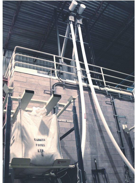
Flexible screw conveyors elevate salt and whey to a height of 30 ft (9m), they are gravity fed through two diverter valves into the sanitary room.
