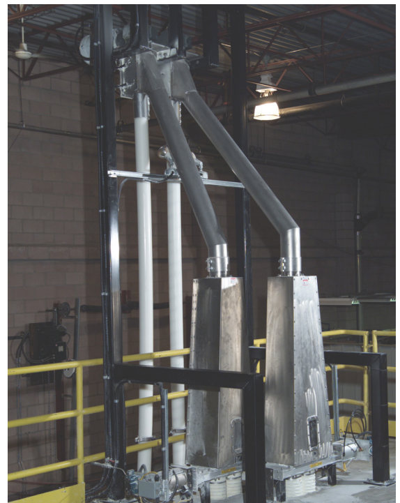
Diverter valves direct salt and whey to either of two raw milk tanks in the sanitary room.
