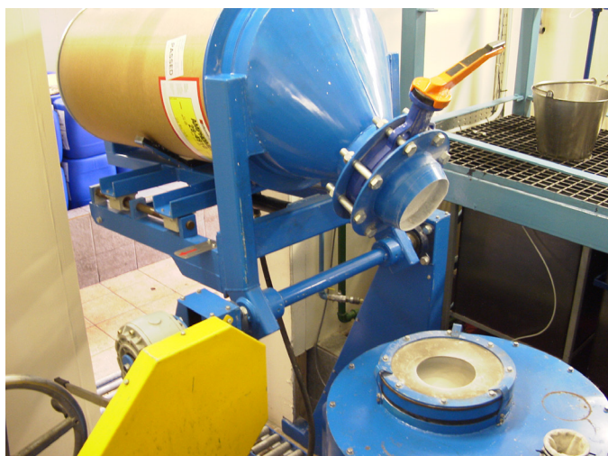
Drum tip approaches point of discharge into 300 gal (130L) capacity receiving hopper
