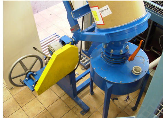
Drum tip engages as neck of butterfly valve is securely positioned against rubber seal on top of receiving hopper.
