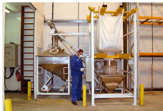
SPOUT-LOCK® clamp ring and pneumatically actuated TELE-TUBE® telescoping tube allow dust-tight connections between bag spout and hopper, and automatic elongation of the bag as it empties for total evacuation of material.
