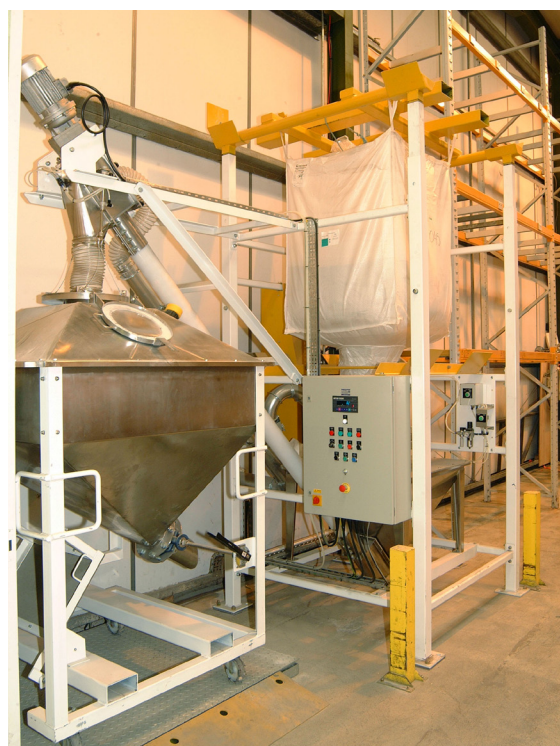
The transfer bin is mounted on a platform scale, which transmits gain-in-weight signals to a controller that runs, slows, and stops the conveyor, achieving rapid batching cycles and +/- 0.04 percent batch weight accuracy.
