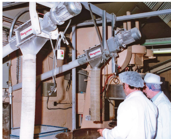
Flexicon added a 7 m long (23 ft) flexible screw conveyor to transfer oatmeal from the discharge station to the mixing area.
