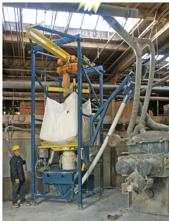
One of three Flexicon bulk bag weigh batch unloading systems equipped with 8 cu ft (226 liter) capacity receiving hoppers and 4.5 in (114 mm) diameter flexible screw conveyors, discharges powder from 2500 lb (1135 kg) bulk bags, transporting it under loss-of-weight control to any of three kneader-extruders. A bag tray support and hinged hopper cover allow manual additions of minor ingredients.
