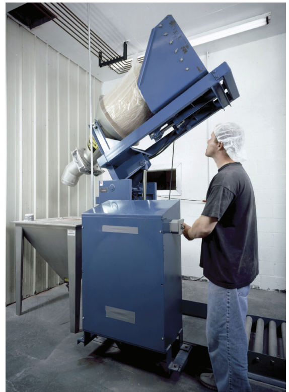
For dust-free dumping, hydraulic lift forms dust-tight seal between drum lip and discharge cone. Discharge cone mates with gasketed receiving ring on hopper lid.
