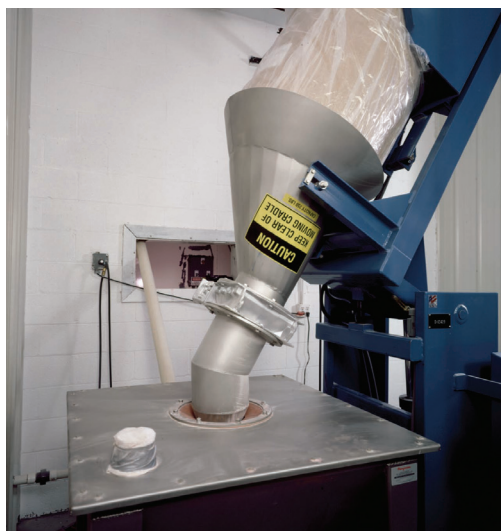
TIP-TITE® drum dumper: Operator controls hydraulic lift which automatically tips drum and mates with receiving ring on hopper.
