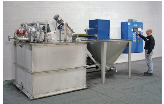
DMax filtration system features an automated dry chemical delivery system that provides more precise dosing than possible with manual methods. A hopper and flexible screw conveyor from Flexicon Corporation deliver dry treatment chemicals to the wastewater holding tank.
