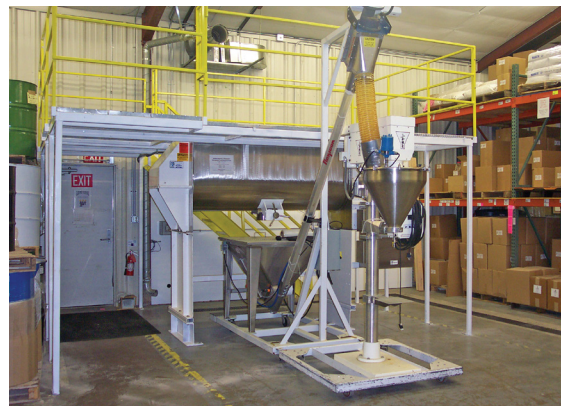
GloryBee utilizes its mobile flexible screw conveyor and mobile filling machine in tandem at multiple plant locations.
