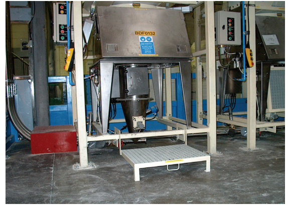
A fold-down step provides access to the telescoping tube assembly, while a dust hood prevents dust emission in the event of a system failure at the point of discharge, or damage to a bag during transportation.
