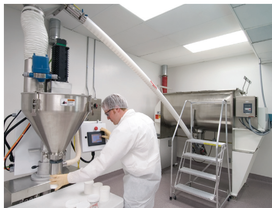
Due to space constraints, Macleod Pharmaceuticals selected a Flexicon flexible screw conveyor to transport powder between a ribbon blender to a filling machine.
