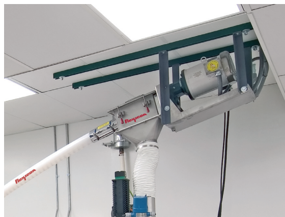
Flexicon engineers maximized the curvature of the conveyor tube and calculated the corresponding angle of the discharge adapter to fit in a low headroom area.
