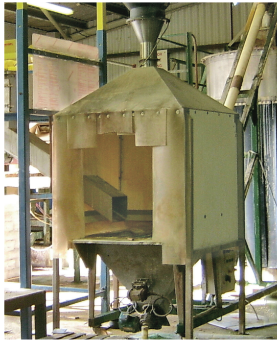
Discharge chute interface with side-mounted vibrator runs from bag outlet to hopper.
