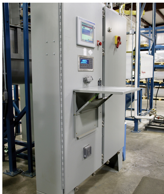
An automated control system manages the entire process according to pre-programmed batch recipes.
