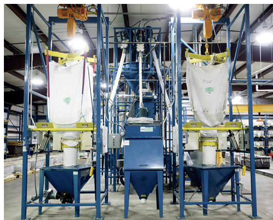
Bulk bag unloaders utilize a proprietary bag-spout interface that creates a high-integrity sealed connection to contain dust and prevent contamination of the product and plant environment. A manual bag dump station with dust collection (center) protects workers and prevents plant contamination.
