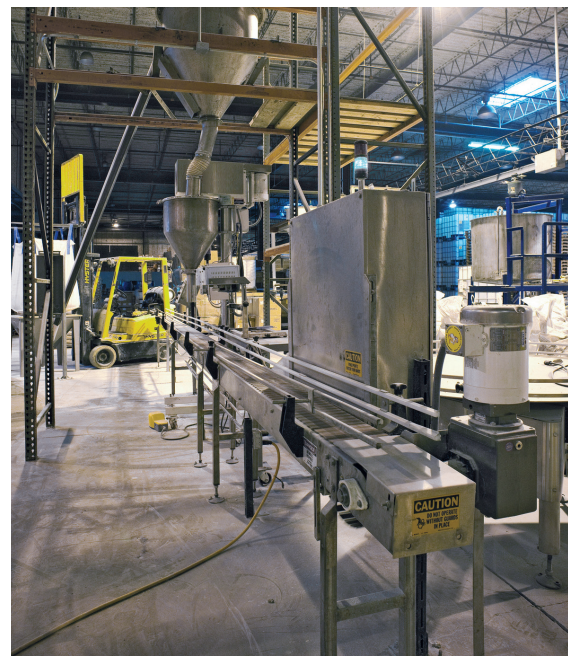
A flexible screw conveyor proved the best way to move the perlite mixture to a ceiling-high surge hopper above the packaging machine.
