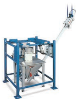
This Half Frame Bulk Bag Discharger offers total dust containment at low cost by eliminating upper frame components to lift and/or position the bag, instead relying on the user's forklift or plant hoist to suspend the bag above the unit during operation.
