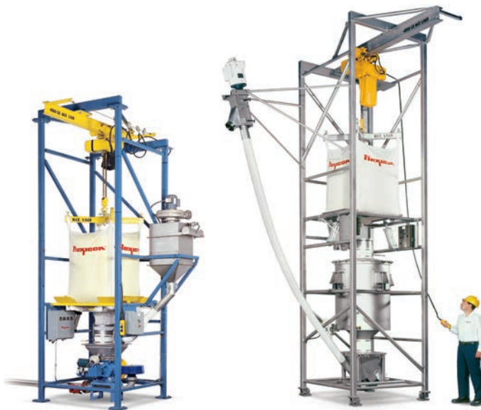
This BFC Series Bulk Bag Discharger is equipped with a small surge hopper that directs material into the throat of a variable speed rotary airlock feeder for volumetric or gravimetric metering into positive- or negative-pressure pneumatic conveyor lines.
